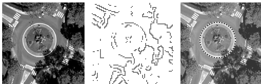
(c) Roundabout with |\mathcal{A}| = 726 . The solution was found in 172.46 seconds and 31,210 iterations.
